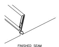
NOTE: STANDARD FACTORY NOTCH IS 1-1/8". LONG LENGTH PANEL INSTALLATIONS REQUIRE GREATER FIELD NOTCHING DEPTH.
