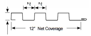
b. 10" rib with 2" reveal, 1.2FX20-12 (1 1/4" rib height) or 1.5FX20-12 (1 1/2" rib height) [select appropriate rib height]
