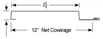
c. 6" consistent rib spacing (6" up / 6" down), 1.2FX30-12 (1 1/4" rib height) or 1.5FX30-12 (1 1/2" rib height) [select appropriate rib height]
