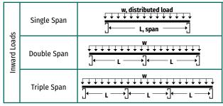
Top values based on allowable stress (ASD). Bottom values based on a deflection limit of L/180.
